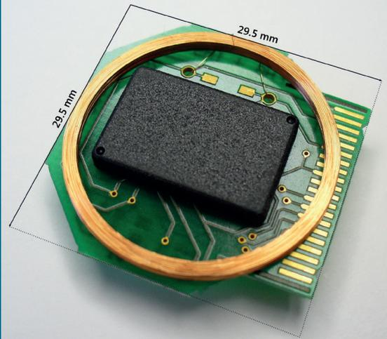
15 cm. As external components for the ASIC, only an antenna based on a coil with a resonance capacitor and an additional capacitor for smoothing the operating voltage are necessary, reducing cost and increasing reliability of the system (Figure 4). The sensor is calibrated in a fully automatic way, storing the calibration coefficients for pressure and temperature in the onchip and system EEPROM.
